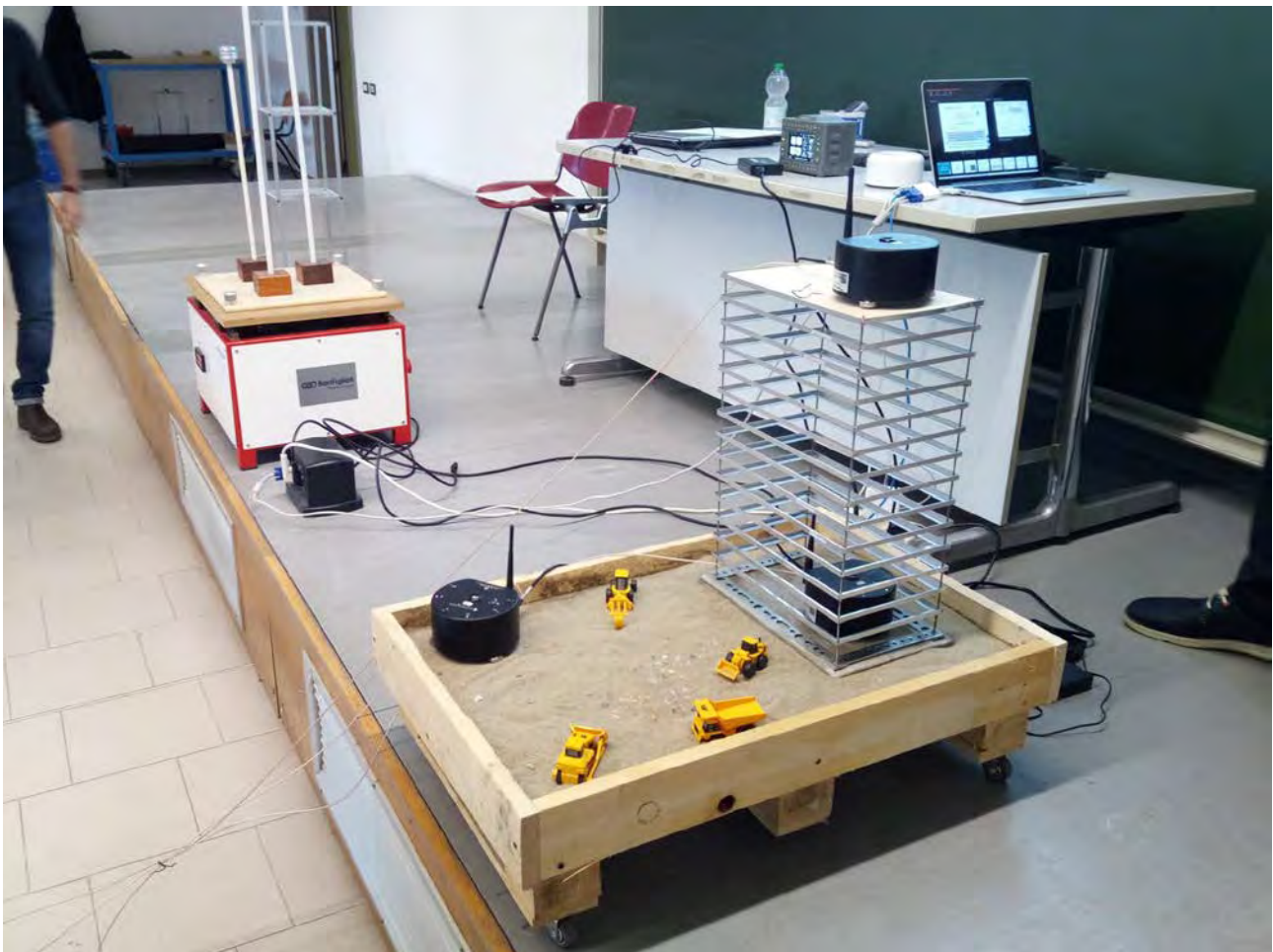
Tests on vibrating table simulating the seismic response of a building.
